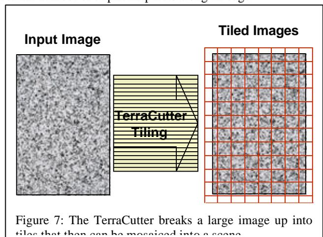
Figure 7: The TerraCutter breaks a large image up into tiles that then can be merged into a scene.
