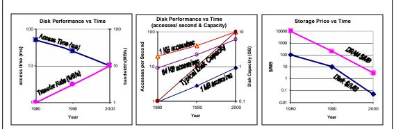
**Figure 1:** Performance of magnetic storage disks over time. The first two graphs show features that improved 10x or 100x while the third graph shows features that improved 10,000x in the same time. The graphs show that access times have improved relatively little, while prices have dropped by a factor of 10,000; unit capacity and accesses per second have grown by a factor of 100. Higher bandwidth and cheaper DRAM buffers have allowed larger pages. That is one theme of this paper.
