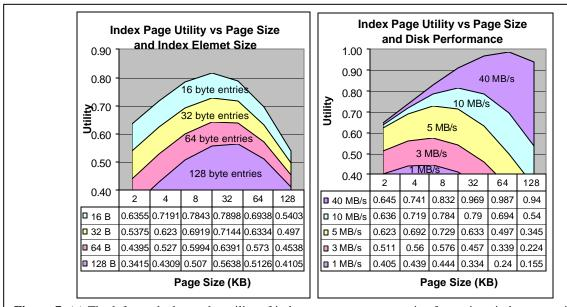
**Figure 7**. (a) The left graph shows the utility of index pages versus page size for various index entry sizes using a high-performance disk (10ms latency, 10 MB/s transfer rate). (b) The graphs at right use a fixed-sized 16-byte entry and show the impact of disk performance on optimal page size. For high-performance disks, the optimum index page size grows from 8KB to 64KB.
