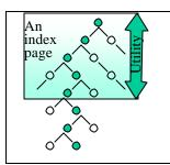
**Figure 5**: The utility of an index page is the number of levels of the binary tree that it traverses. The utility rises as the log of the page size. The cost of the access goes up linearly with page size. Consequently, for a particular disk latency and transfer rate, there is an optimal index page size. The tree at left shows just the search path (it is not balanced because the drawing would be too cluttered)
